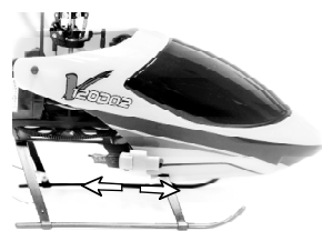
Step 1: disconnect the power cable of helicopter.
