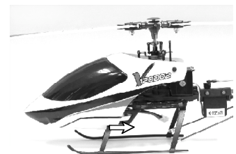
Step 3: take off the canopy and remove the battery pack.
