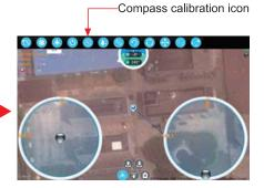
**IMPORTANT:** Make sure the motors are locked before calibration (Aircraft red LED indicator is NOT flashing). Factory default setting, is for the motors to be locked after the completed ID binding process. (For details on motor lock and unlock process see point 10 and 11)
