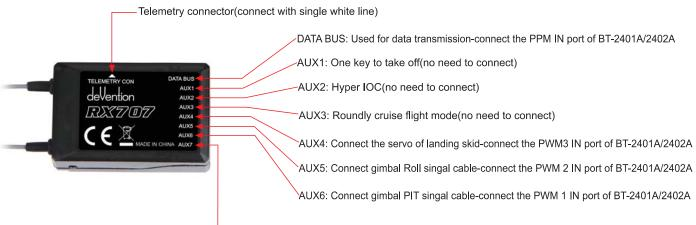
AUX7: Connect camera controller/Clear fix ID code(When clear fix ID code is need, insert random equipped bind plug pls).
