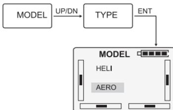
Press UP or DN to select AERO, Press ENT to confirm and then press EXT to return to MODEL.
