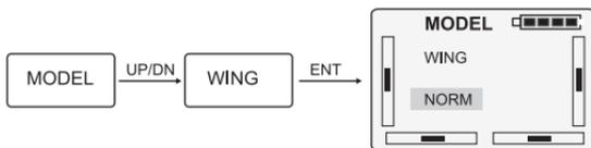
Press R or L to select NORM, Press ENT to confirm and then press EXT to return to MODEL.
