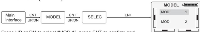
Press UP or DN to select "MOD 1", press ENT to confirm and then press EXT to return to MODEL.
