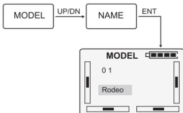
Press R or L button to change the character and figure, named model as Rodeo. Press ENT to confirm and then press EXT to return to MODEL.
