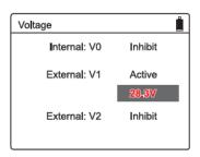
Internal shows the Radio battery voltage.
