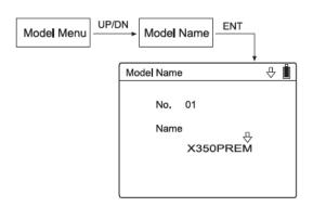
Press UP or DN button to select the characters which need to be changed, Name model "X350PREM".
