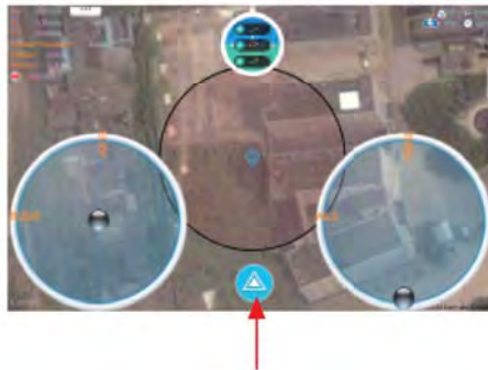
Long press stable mode icon: Motor unlocked
